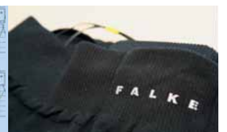
Contractions of leg muscles are measured and transmitted to a computer for individual analysis.
